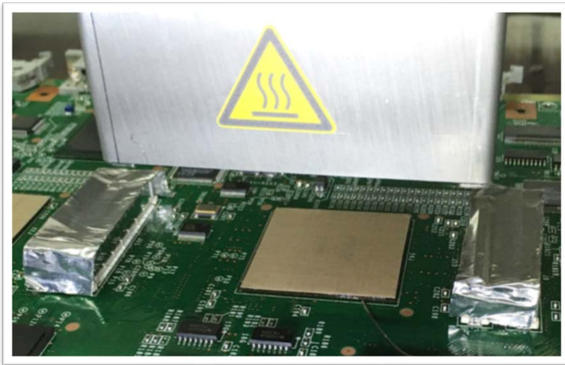
Figure 6: Tin Foil on Adjacent Parts for Ceramic IR Heating
